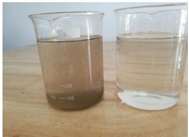
Influent (Left) & Effluent (Right) of AMSFS II 磁介质高效沉淀池的进水 (左) 和出水 (右)
