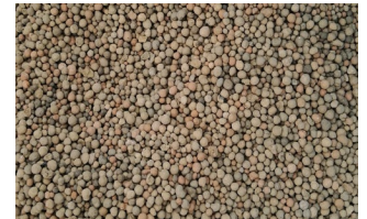
Filter media made of natural clay 黏土制成的滤料
