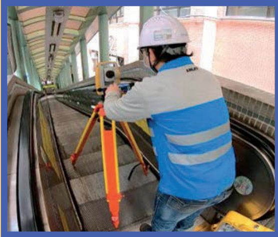
Accurate data about the escalator was obtained through TS, a tool not normally used in our industry.
